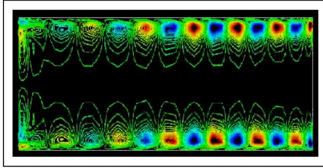
Figure 4. Axisymmetric time-dependent instability in the annular rotating cavity ( $R_m = 5$ ,  $L = 3.37$ ) for  $Re = 1750$  and  $C_w = 530$ . Iso-lines of the fluctuation of the axial velocity in the plane  $(r, z, \pi/4)$ . Animation available on the IJFD website.
