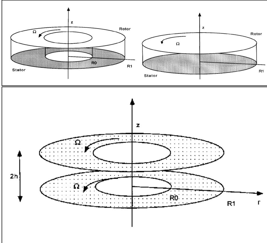
Figure 1. Geometric models. (a) Top left: annular rotor-stator cavity, (b) Top right: cylindrical rotor-stator cavity ( $R_0 = 0$ ), (c) Bottom: rotating annular cavity with a radial outflow.
