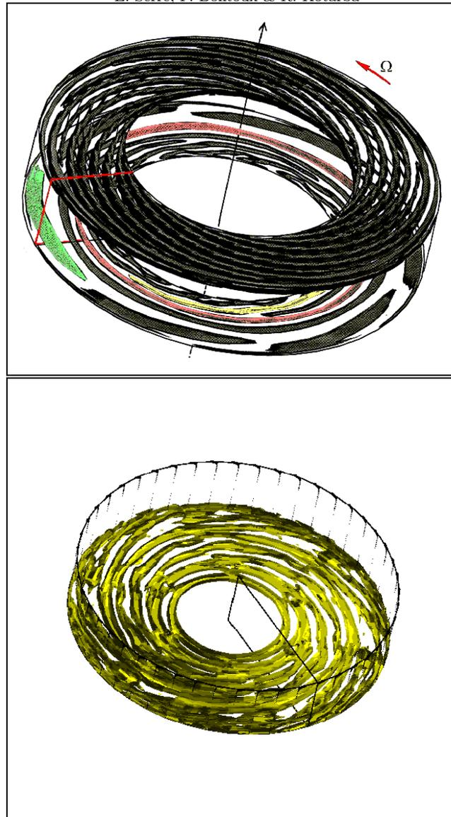
Figure 3. Mixed annular and spiral patterns of the instability in the rotor-stator cavity. Three-dimensional display of iso-surfaces of the fluctuation of the axial velocity component. (a) Top: Ekman and Bödewadt layers instability in the annular cavity ( $R_m = 5$ ,  $L = 5$ ,  $Re = 330$ ). The annular structure is colored pink and the spiral arms are colored in yellow and green close to the shaft. (b) Bottom: Cylindrical cavity ( $L = 5$ ,  $Re = 1200$ ).
