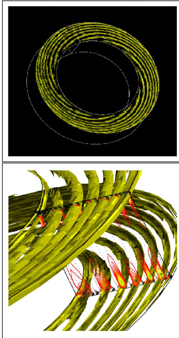
Figure 5. Spiral patterns ( $n = 12$  arms) of the Ekman layer instability. Three-dimensional display of iso-surfaces of the axial velocity component in the annular rotating cavity ( $R_m = 5$ ,  $L = 3.37$ ) for  $C_w = 530$  and  $Re = 1750$ . (a) Top: Spiral patterns in the upper Ekman layer; an animation is available on the IJFD website. (b) Spiral patterns in both Ekman layers (yellow), velocity field and contours of positive axial velocity in a  $(r, z)$  meridional plane.
