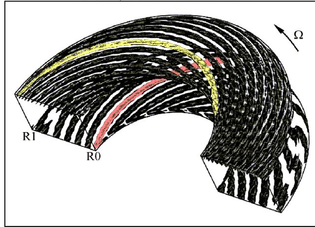
Figure 2. Spiral patterns of the instability in the rotor-stator cavity. Three-dimensional display of iso-surfaces of the fluctuation of the axial velocity component: (a) Ekman and Bödewadt layers instability (yellow and pink arms, respectively) in the annular cavity ( $R_m = 5$ ,  $L = 5$ ),  $Re = 330$ .
