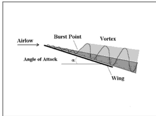
Figure 1. Representation of vortex bursting over a delta wing.
