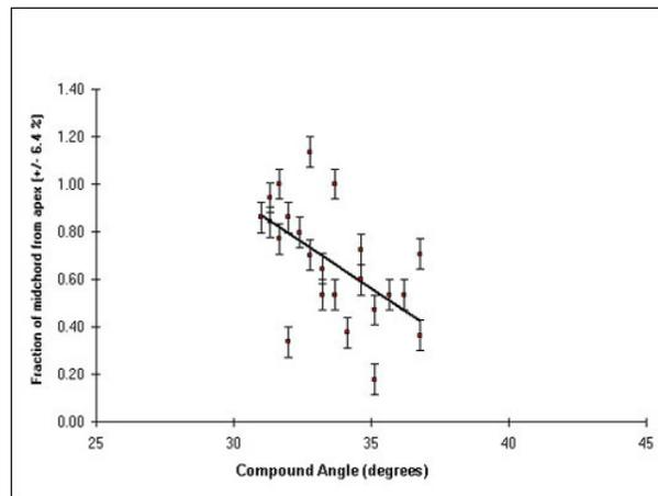
Figure 8. Burst point as a function of compound angle.
