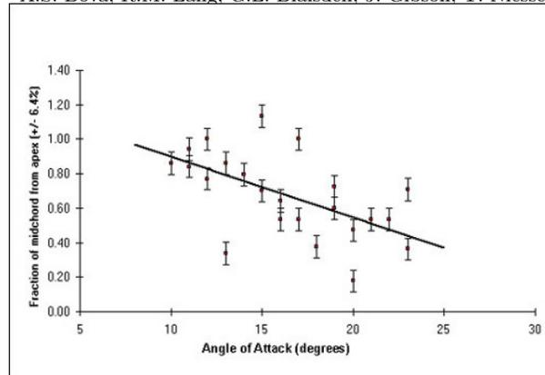
Figure 7. Burst point as a function of angle of attack.
