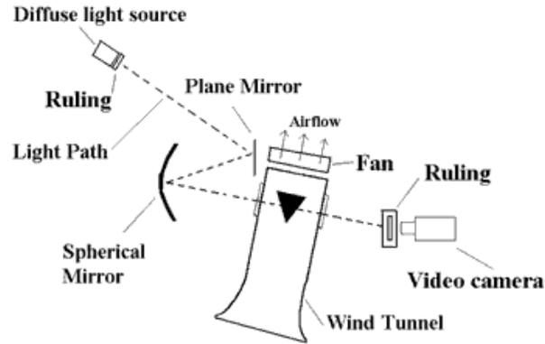
Figure 3. Schlieren optical arrangement. The source light was 2.3 m from the plane mirror, the plane mirror was 0.7 m from the spherical mirror. The distance from the spherical mirror to the camera's objective was its focal length, 3 m. The angle between the source light and the normal to the plane mirror surface was 20 degrees
