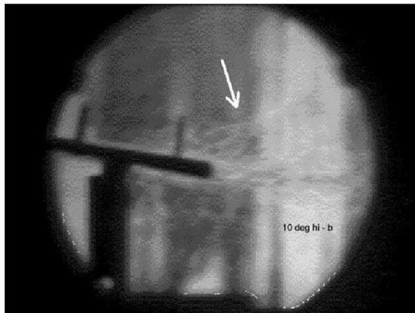
Figure 6. Spiral breakdown and vortex bursting at  $10^\circ$  angle of attack. The screws perpendicular to the plane of the wing are 5.1 cm apart. Arrow indicates location of burst point.
