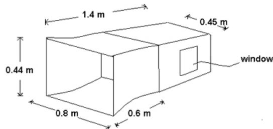
Figure 4. Sketch of the wind tunnel.
