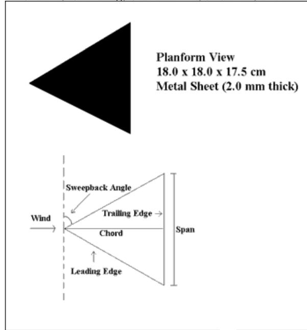
Figure 2. Planform view and wing specifications.
