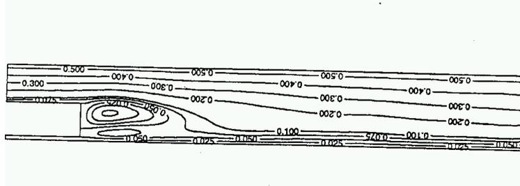
Figure 2. Average streamlines ( $\Gamma = 0.0033$ ,  $\Delta t = 0.05$   $h = 0.05$  and  $Re = 7000$ ; thick bluff-body).
