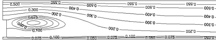
Figure 8. Average streamlines ( $V_j/V_e = 2.0$ ,  $\Gamma = 0.0033$ ,  $\Delta t = 0.025$ ,  $h = 0.05$ ,  $Re = 7000$ ; thick bluff body)
