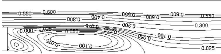
Figure 7. Average streamlines ( $V_j/V_e = 0.5$ ,  $\Gamma = 0.0033$ ,  $\Delta t = 0.025$ ,  $h = 0.05$ ,  $Re = 7000$ ; thick bluff body)
