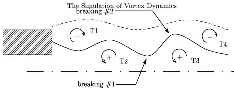
Figure 3. Eddy formation mechanism ( $\Gamma = 0.0033$ ,  $\Delta t = 0.05$   $h = 0.05$  and  $Re = 7000$ ; thick bluff-body).
