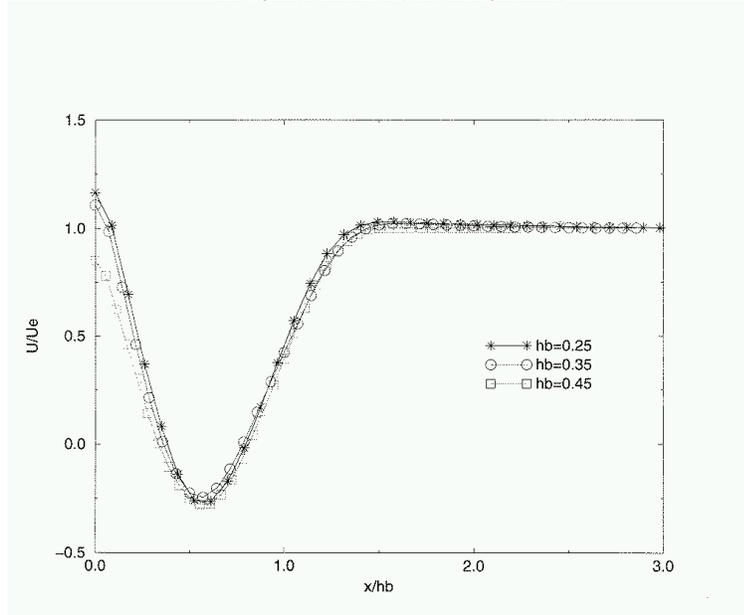
Figure 6. Normalised averaged streamwise velocity profiles  $U/V_e = f(y/h_b)$  for the three bluff-bodies for the same relative distance  $x/h_b$  from the bluff-body base.
