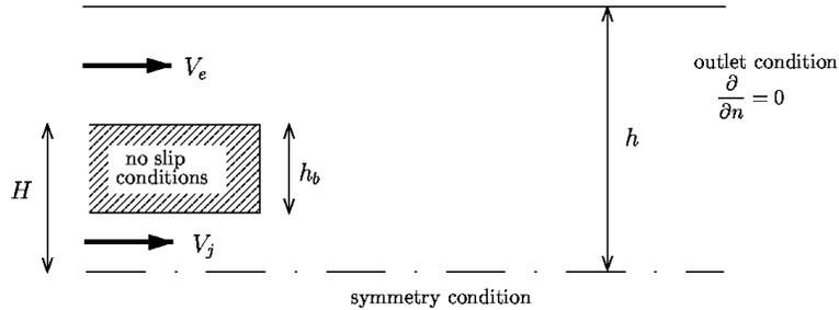
Figure 1. Geometry of flow domain showing boundary conditions
