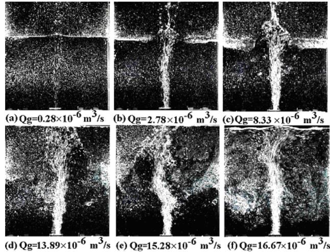
Figure 2. Samples of the recorded images at various gas volume flow rates.
