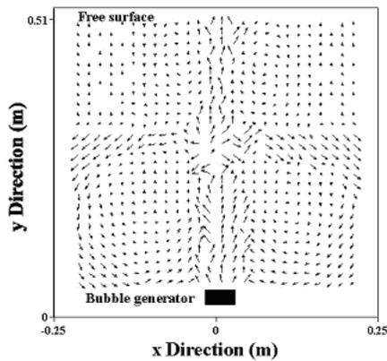
Figure 4. Velocity vector map of the flow pattern for  $Q_g = 0.28 \times 10^{-6} \text{ m}^3/\text{s}$ .
