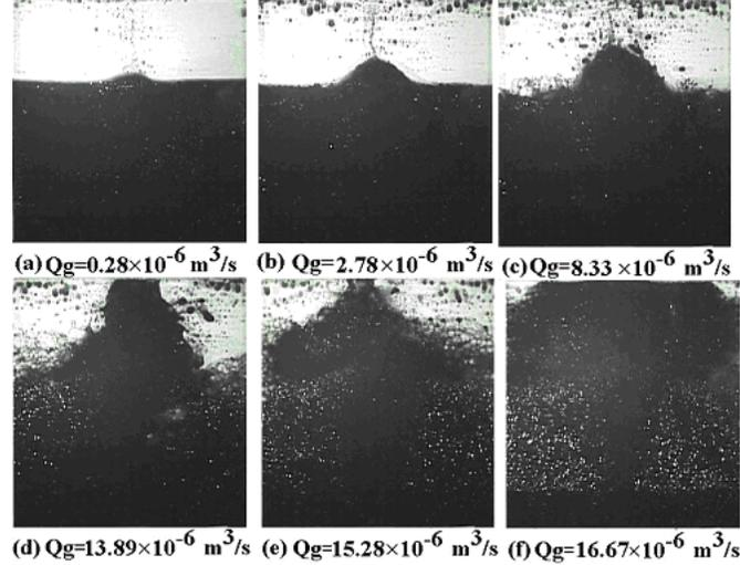
Figure 7. Phase distributions versus gas volume flow rate.
