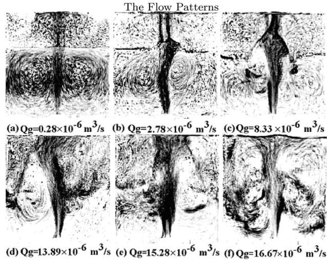
Figure 3. The pathlines of the flow pattern at various gas volume flow rates.
