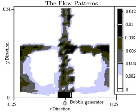
Figure 6. The kinetic energy  $(\text{m/s})^2$  for  $Q_g = 0.28 \times 10^{-6} \text{ m}^3/\text{s}$ .
