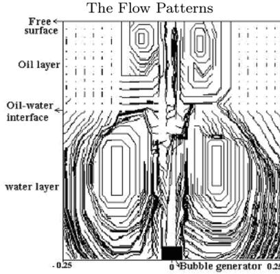
Figure 5. Streamlines obtained by PIV for  $Q_g = 0.28 \times 10^{-6} \text{ m}^3/\text{s}$ .
