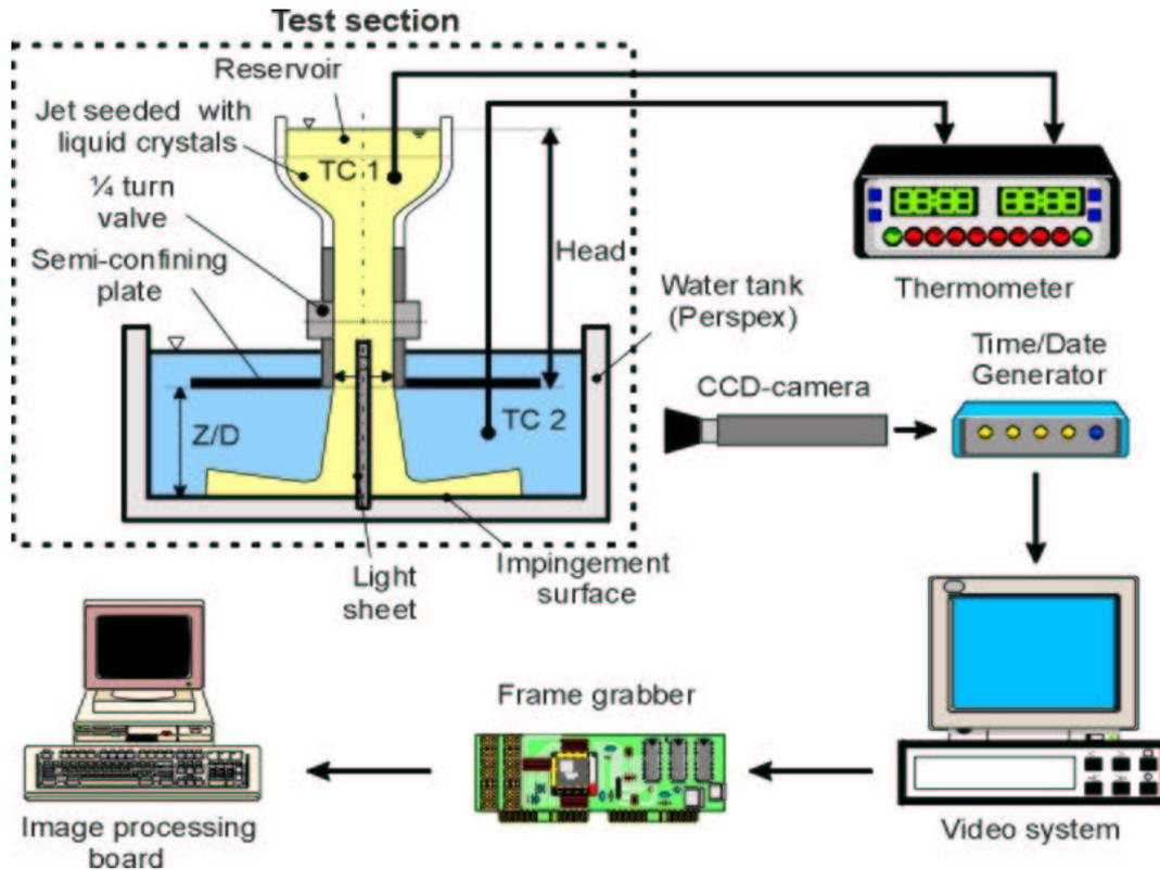
Figure 1. Schematic of the experimental rig and data collection and processing.
