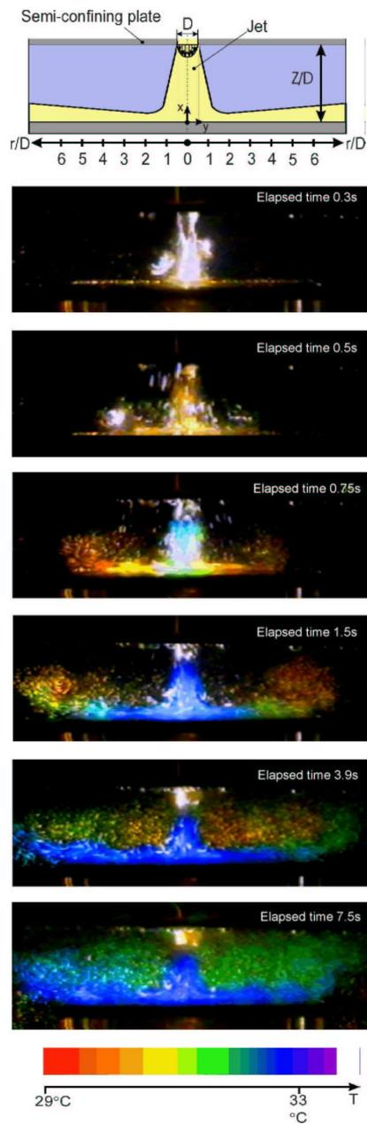
Figure 2. Still images of the flow at different time showing thermal field.
